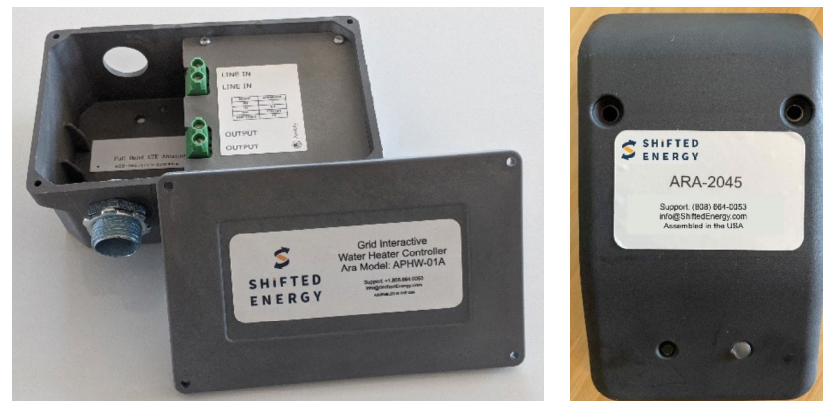
Shifted Energy's load control switches are IoT devices designed for interoperability across electric water heater technologies and products.
