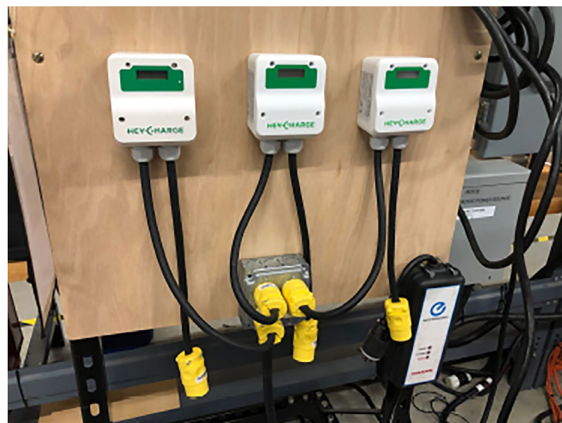
At EPRI’s EV laboratory, three HeyCharge access points with Bluetooth capability were deployed and tested for app-based, end-to-end management of the EV charging process.
