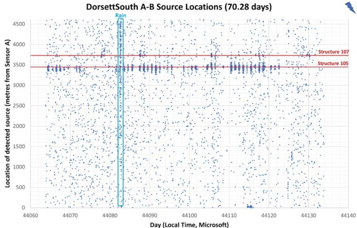
*EFD chart showing intermittent partial discharge activity at an 138kV insulator string on Phase A, Structure 105*
